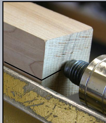
Mount between centers and transfer the angle line to the opposite end of the blank
