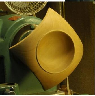
Hollow out the bowl being careful to leave the rim intact. Sand to your final grit and if you are going to apply finish on the lathe, then do it now.
