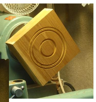
Round off the top being careful to not go over the edge (leave the corners of the block). If your wood has a tendency to chip try soaking the edges with Cyanoacrylate glue.
