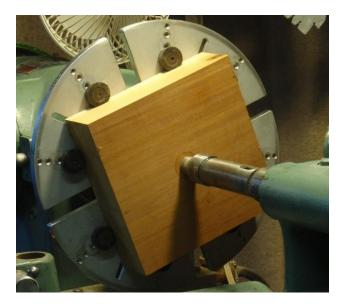
Clean up and flatten the bottom, then cut a 2 inch (ID) by 2 3/4 inch circular groove, make sure the groove is wide enough for your #2 jaws. Using the jumbo jaws to create the tenon will ensure it is exactly centered on your blank.
