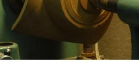
Remove the bowl and remount the top so the underside can be shaped. Sand to your final finish and, again if you are going to apply finish on the lathe, now is a good time to do that. Remount your bowl and using it as a jam-chuck shape the top so that the bowl and top appear to be a continuous curve. Leave a tenon so the piece can be reversed.
