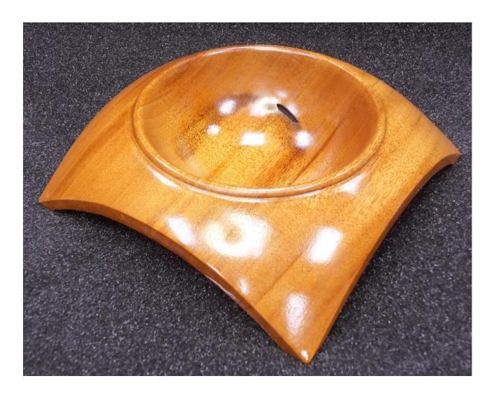
January, 2015 Clifford C. Weatherell Start with a square block of wood, try to pick a species with tight grain that will turn well. Mount the block, in your jumbo jaws, with the bottom of your bowl toward the tail stock. I like to use my tail stock to hold the block in place while I tighten the chuck to ensure the block is tight against the jaws.
