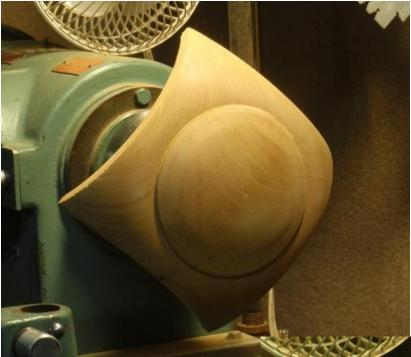
Remove the top and remount the bowl. Once again using the bowl as a jamchuck turn the tenon off the top and sand to your finish grit. If you are going to apply finish on the lathe, now is a good time to do that.
