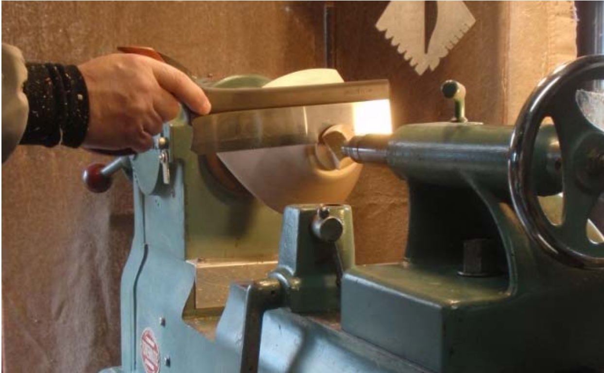
A saw is used to remove the last bit of the point that was in the live center.
