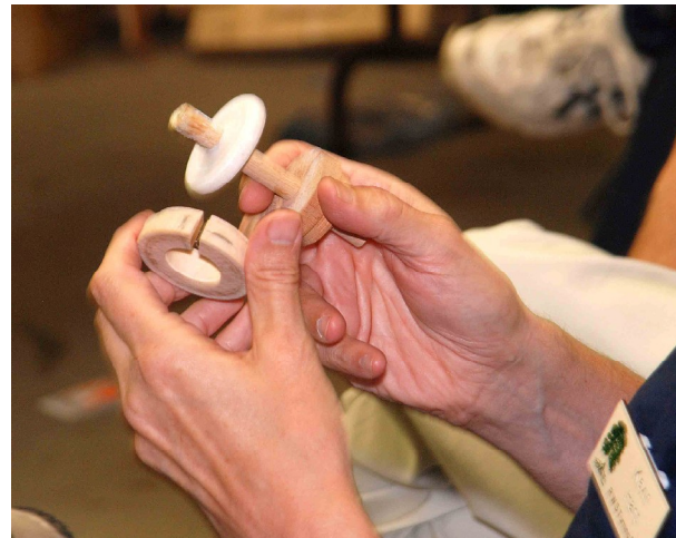
To right: Mike demonstrates a very clever method of scroll chucking a dowel without marring it, by making a round, split wooden insert, which, when tightened in the chuck, grips the dowel securely without damage.
