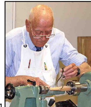
Bill uses calipers to gauge part
