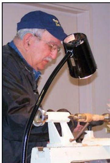
Turning a refrigerator magnet<sup>1</sup>
