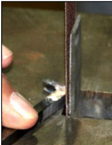
Tool shaped on a wheel or belt grinder to eliminate sharp corners<sup>1</sup>
