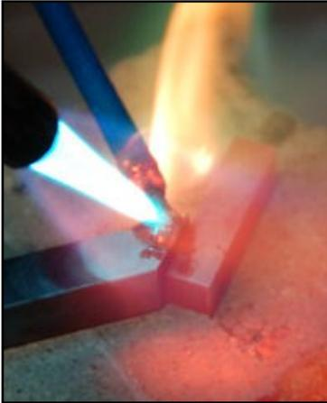
Shank and cutter heated to a bright red color and silver soldered<sup>2</sup>
