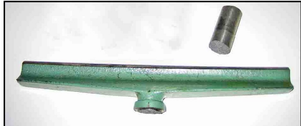
Jim's broken tool rest. (As a courtesy to the squeamish, we're not showing photos of Jim's finger!)
