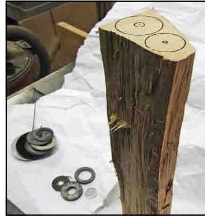
Jim uses a variety of different diameter washers to lay out dowel stock
