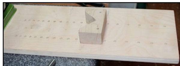
Base for holding lathe tool for sharpening
