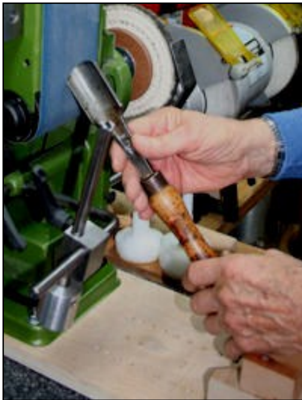
Sharpening a conventional gouge
