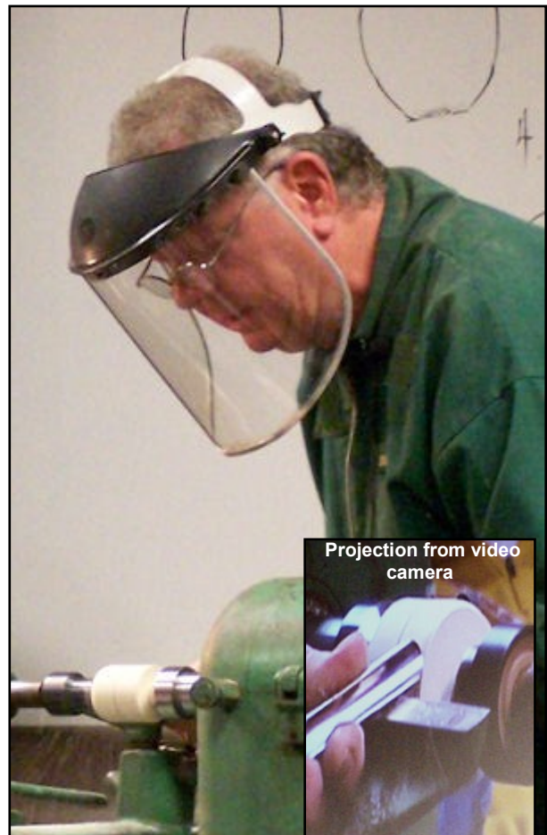
Turning the outside of the ornament globe with a spindle gouge
