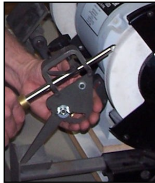
Sharpening a spindle gouge
