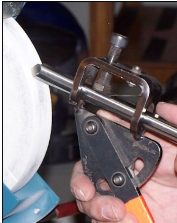
Sharpening a side grind bowl gouge
