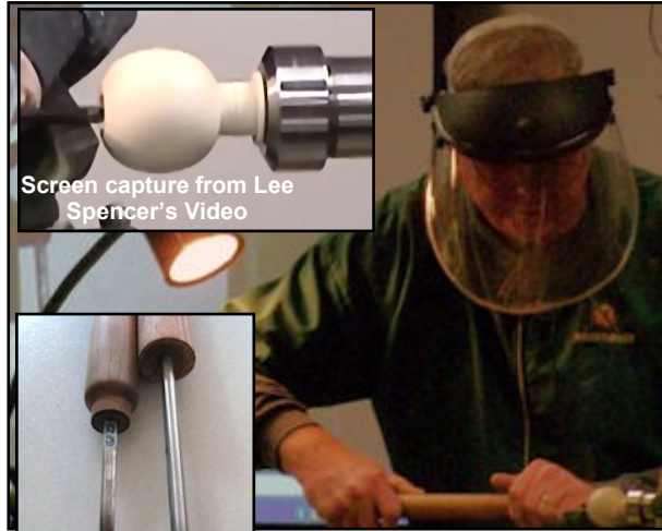
Hollowing the Ornament. The top inset shows a clearer view of Bruce hollowing the ball part for an ornament. The work is held with a Beall Collet Chuck.
