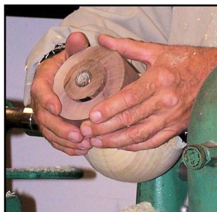
Fitting head stock cup to rough turned sphere
