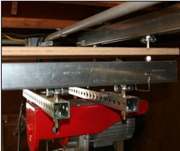
Figure 4. Picture of Hoist and Rail Connections
