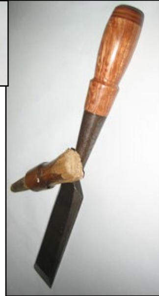
**New handle on refurbished chisel.**
