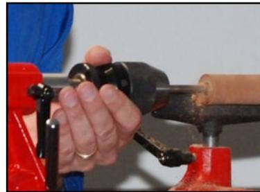
Drilling the 1/2" hole for the needle box lid.
