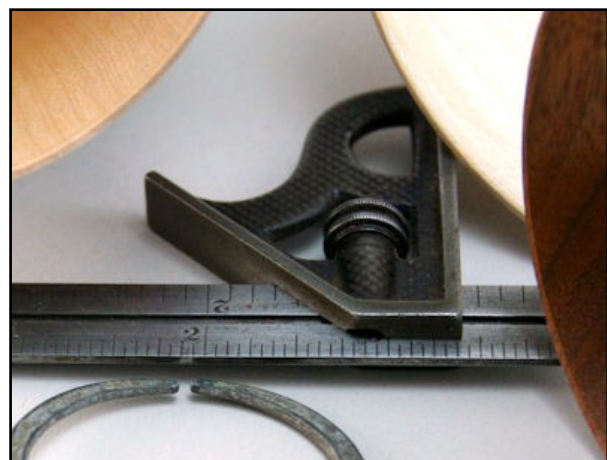
Measurement showing walls are 1/16 inch thick
