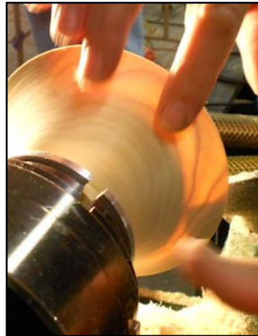
Back light showing thin wall
