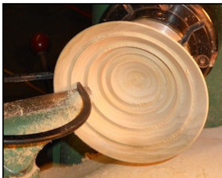
Measuring the wall thickness
