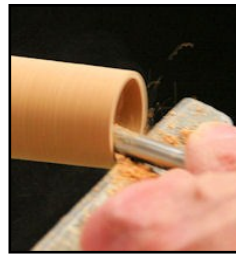
11. Tapering the inside of the candle holder cup to fit the base of a candle.
