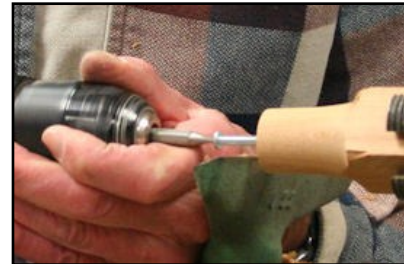
21. Screwing the 8-32 machine screw into the 9/64" center hole.
