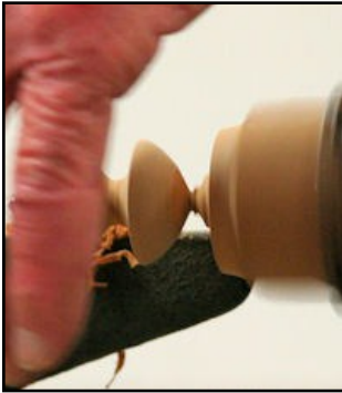
26. Parting off the knob. Leaving a nub to prevent fibers from pulling out.
