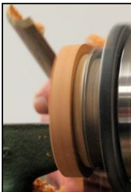
29. Mounting the top in a chuck
