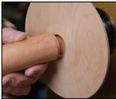
38. Detail showing the fitting of the candle holder body to its base.
