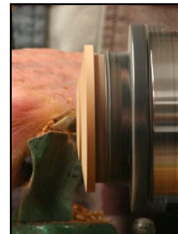
32. Finishing the bottom of the cup.
