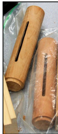
6. Finished Candle Holder body with slot and 1/4" tenon on the bottom.
