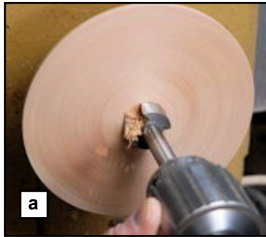
37. Turn the base to a diameter of 6", drill 1 1/8" diameter recess to a depth of 1/4" and finish.
