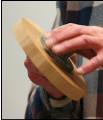
36. Mount to a faceplate a 13/16" X 6 1/4" square block.
