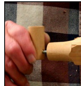
23. A check to assure the cup handle is square with the cup.
