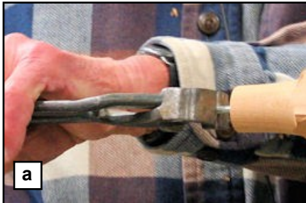
22. Cutting the head off the machine screw and removing the burr.
