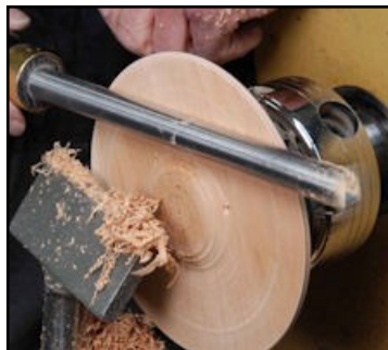
39. Re-mounting the base in a chuck to finish its bottom.
