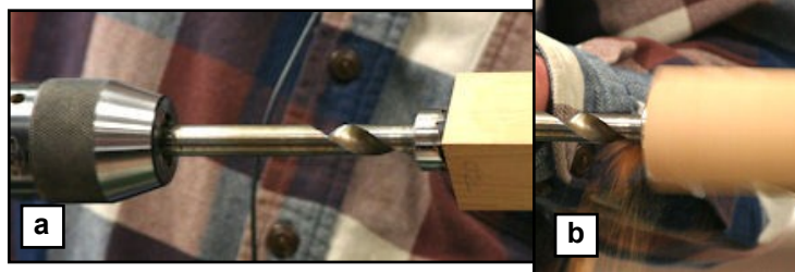
2. Boring a 1" diameter hole in the candle holder body
