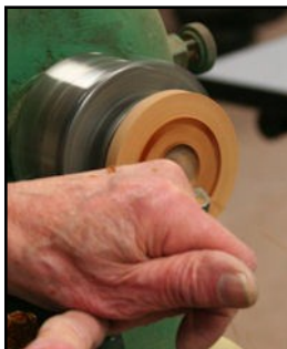
33. Reverse on chuck and finishing the cup top.
