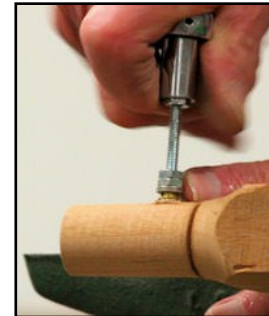
15. Removing the insertion tool.
