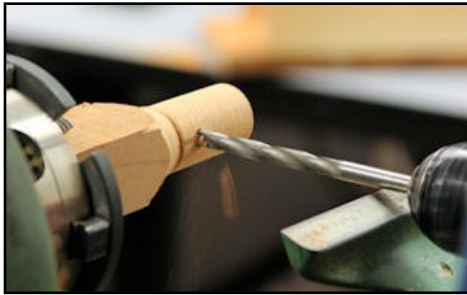
13. Drilling a 17/64" hole in the candle holder cup to receive an 8-32 threaded brass insert. This insert is for a handle to raise or lower the candle holder cup within the candle holder body.
