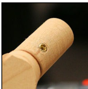
16. Candle holder cup with brass insert.
