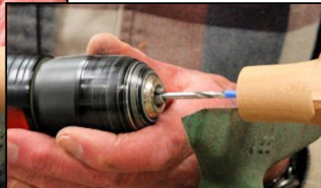
19. Locating the center of the remaining 1 1/8" square x 3" stock. This will be used to make the cup handle.
