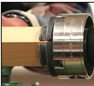
1. Mounting a 1 1/2" square by 7" blank candle holder body in the scroll chuck
