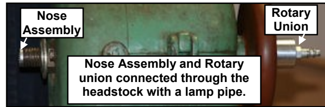
System to transfer vacuum through headstock.
