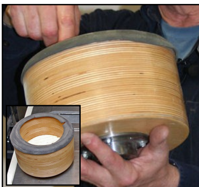
Cup shaped chuck made from laminated plywood. Inset image shows the top and inside of the cup.
