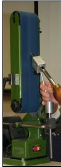
Ward Donahue demonstrating a bowl gouge sharpening jig.
