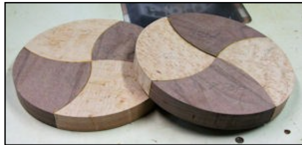
Segments glued together after dry fitting.
