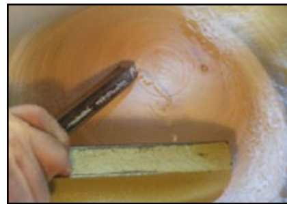
Final interior finishing cut.*
