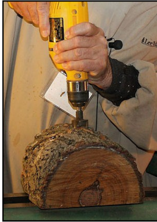
Removing bark with a multi-spur drill bit.
