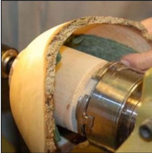
Holding the bowl with a padded waste block to finish the base.*
