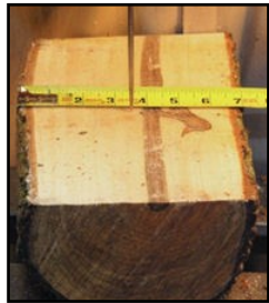
Mark centers side to side and end to end.
