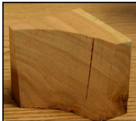
Bill McColgin A turning from 45° Wood (Not face grain, not end grain) From the corner of a bowl blank
