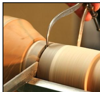
Parting cut to mark final depth
