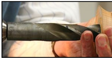
Use the 1 inch drill bit to clean the glue joint
