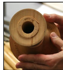
Parting off the top waste block exposing the hole for the glass tube
