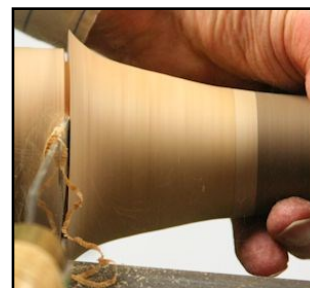
Parting off the top waste block exposing the hole for the glass tube
