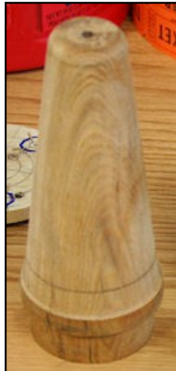
Hardwood form for molding the horn
