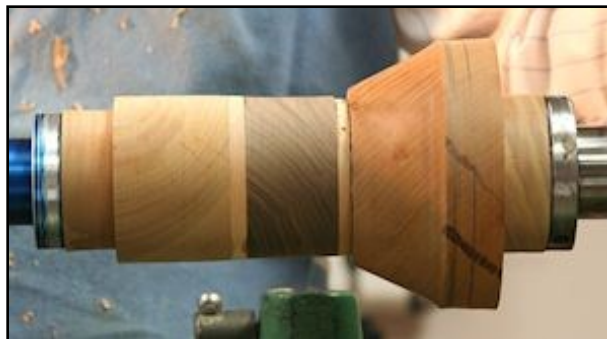
A previously assembled segmented vase turning blank
