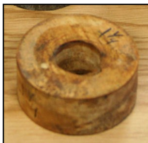
Wood doughnut to push the horn on the wood form
