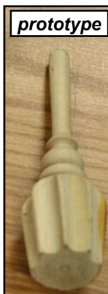
Curly maple stir rod treated with a dye and finished with heat treated linseed oil
