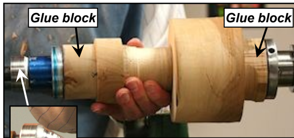
Top and bottom segments glued together
