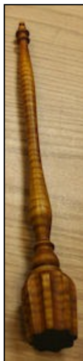
Curly maple stir rod treated with a dye and finished with heat treated linseed oil
