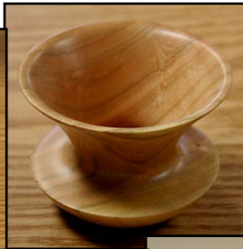
Bill McColgin A turning from 45° Wood (Not face grain, not end grain) From the corner of a bowl blank
