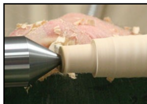
Turning and measuring the handle tenon
