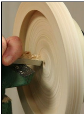
Using a square nose scraper to smooth the bottom
