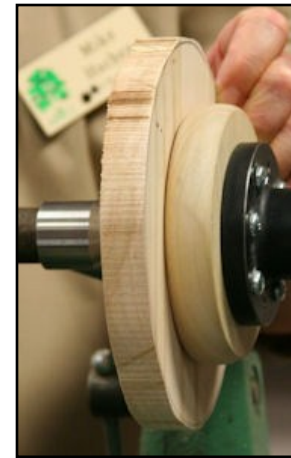
Mounting the mirror base on the waste block with the aid of the tail stock to center and support the work
