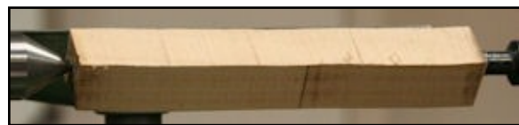
Handle blank mounted between centers
