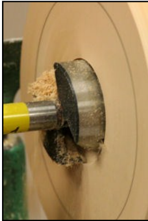
Drilling with the 2 1/8 inch Forstner Bit
