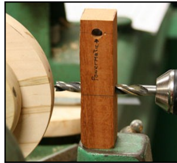
Jig to drill 3/8" hole in the side of the disk to accept the handle
