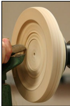
Increasing the recess opening with a bowl gouge
