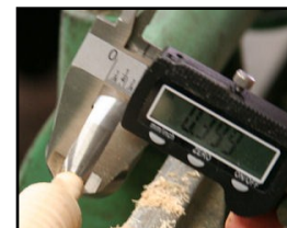
Turning and measuring the handle tenon
