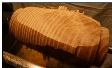
Turn round with tenon on each end
