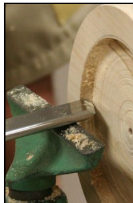
Creating a shallow trough for the silicone adhesive
