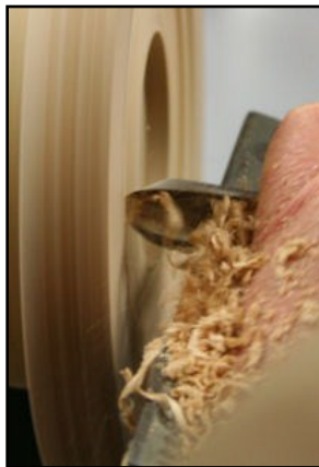
Mirror holder Cross grain turning
