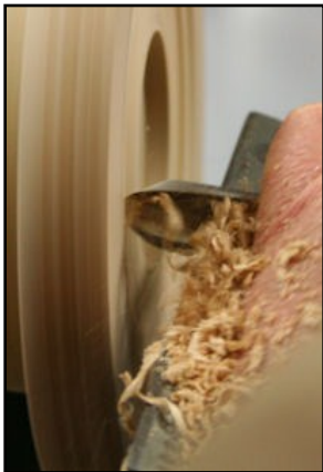
Increasing the recess opening with a bowl gouge
