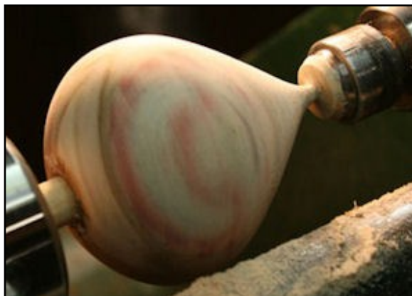
Turning the 2 1/2 x 2 1/2 block to a top shape
