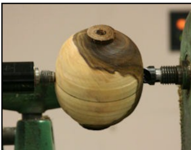
Rotate orientation by 90° Locate centers on pencil line
