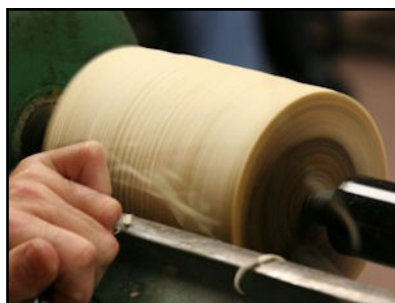
Rough out log between centers with grain aligned with the axis of rotation
