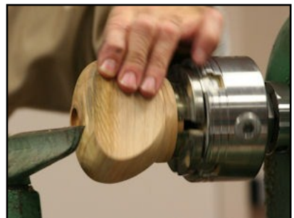
Example with cutaway to show hollowing progress
