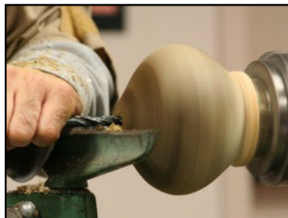
Drill a depth hole
