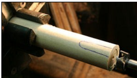
Drilling the center of the 1 1/4" dowel to a depth of 2 1/2"
