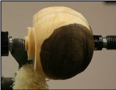
Create a tenon for chucking
