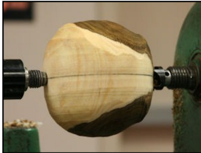
Align pith points straight across by shifting centers away from center line
