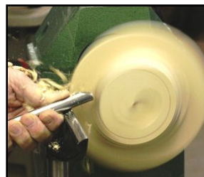
Cut to foot diameter
