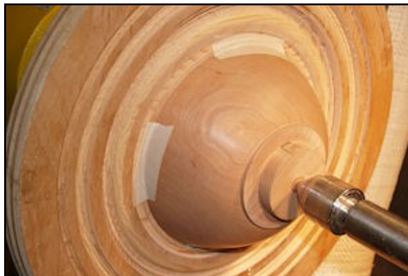
Plywood jam-chuck for finishing the foot
