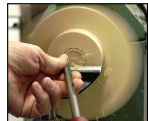
Cut off original recess and cut new one
