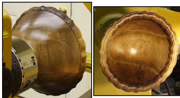
Top and side view of the rim after the bowl was turned, sanded and finish was applied
