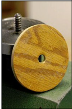
Mount in screw chuck with spacer to reduce depth
