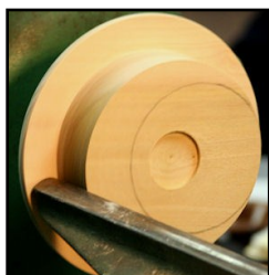
Draw foot diameter from offset hole
