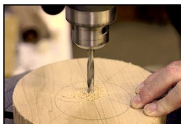
Drill the center hole
