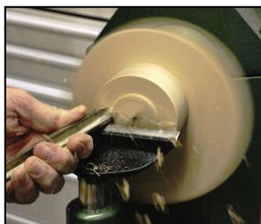
Cut off original recess and cut new one
