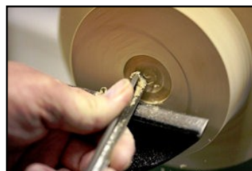
Cut expansion chuck recess on the top.
