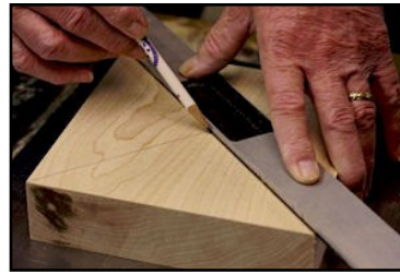
Mark the center on both sides
