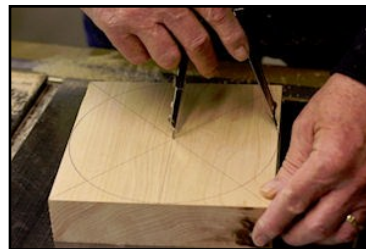
Mark the overall diameter
