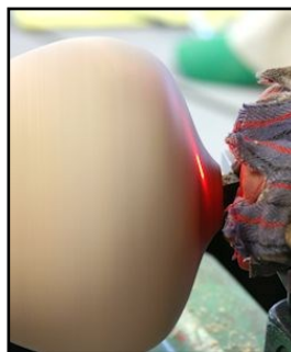
Laser is positioned the desired wall thickness away from the cutting tool
