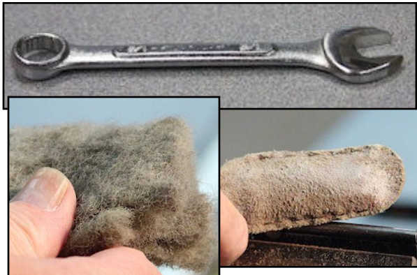
A few of the many tools used by Bruce: sharpened open end wrench for sizing the finial onion, Leather finger protection and a Mirlon pad for fine sanding.
