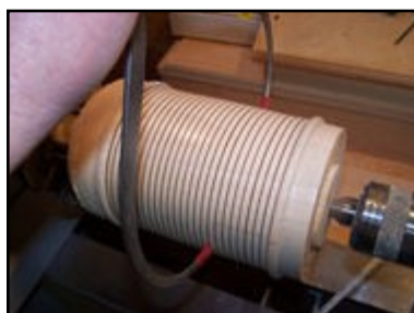
Figure 11 Measuring the diameter of the cylinder.
