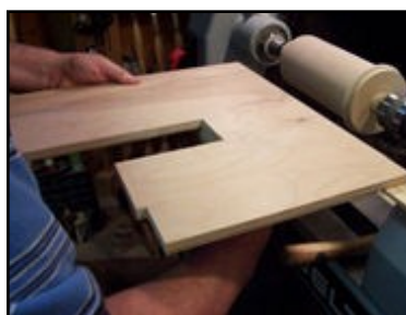
Figure 19 Table top with a straight edge is placed next to the cylindrical turned object.
