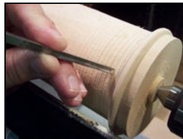
Figure 15 The column location is defined by the tip of the beading tool.
