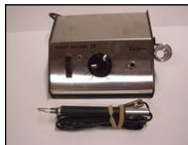
Figure 22 The Wood Burning Equipment used to burn the column lines.
