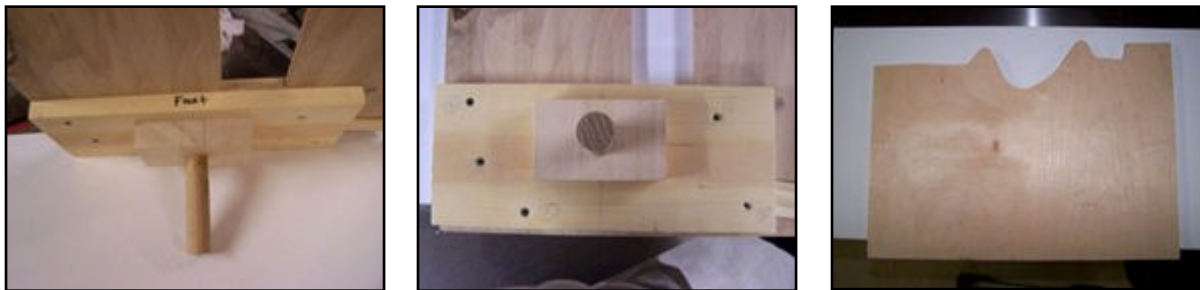
Figure 18 Three different views for the table used to draw in the lines to define the columns. The photo on the left is a side view of the table. The middle photo shows the permanent bottom assembly. The photo on the right shows a replaceable top.
