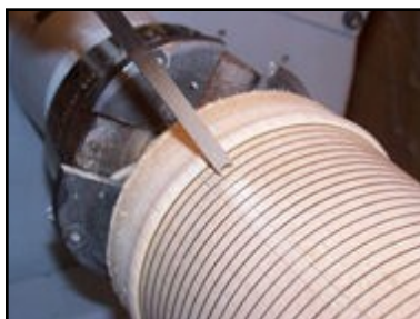
Figure 14 Defining the column location with the tips of the beading tool.
