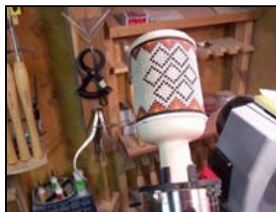
Figure 27 Photo sequence for the coloring of the diamond pattern on the turned object. The brown edge pattern was completed.
