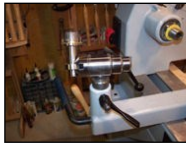
Figure 21 Photo of chuck holder held in the tool rest used during the wood burning process.
