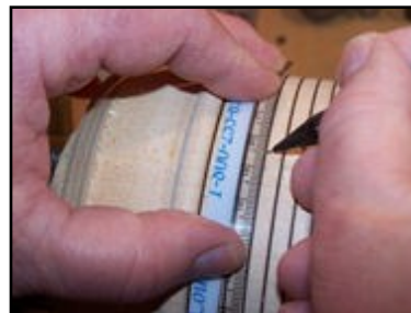
Figure 16 Marking the location for each column with a flexible measuring tape and pencil.
