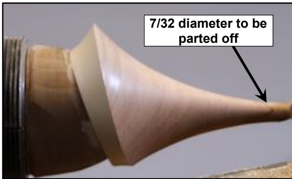
Turned base before removing from the chuck
