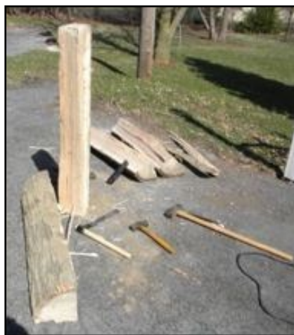
Riving the log using a tools
