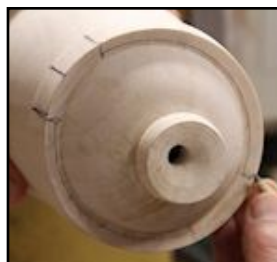
Marking the handle location and rim carving depth
