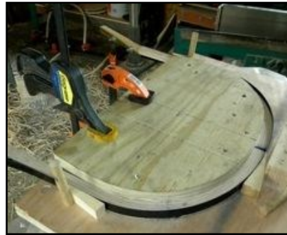
Steam bending form with chair arm cooling down. Notice the metal strap which helps avoid grain from separating
