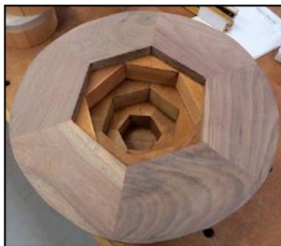
Figure 7 Staggered Nature of Glued-Up Stack
