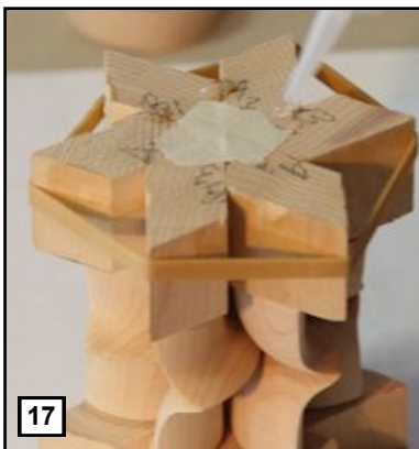
17 Assembling, gluing and clamping the six turnings
