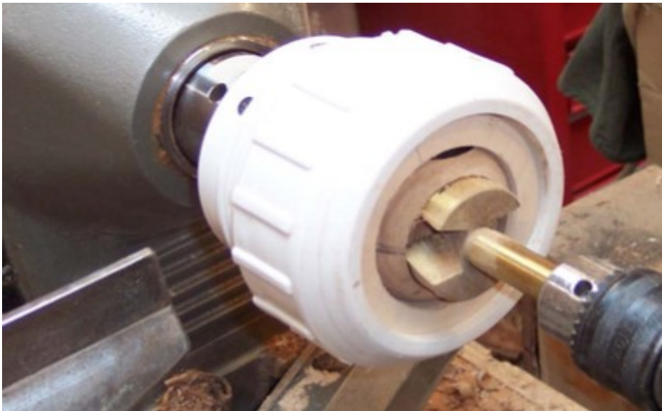
Picture 4: By drilling two adjacent holes, you can check to ensure that you are drilling to the proper depth to obtain the optimal overlap of the holes to create the effect of cubes.
