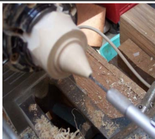
Photo 7. Drilling the \frac{3}{32} " hole in the cone
