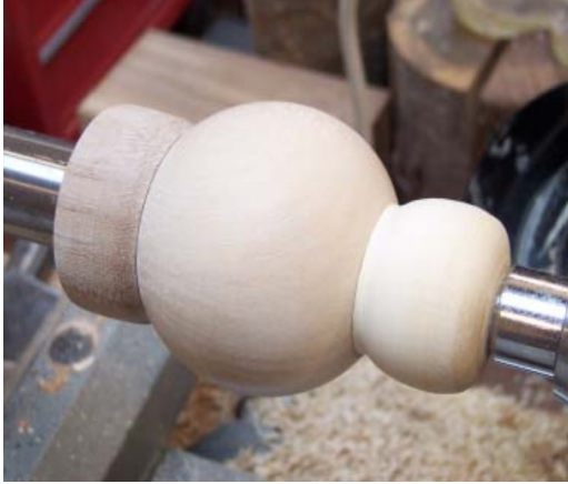
Photo 10. Between centers for Sanding
