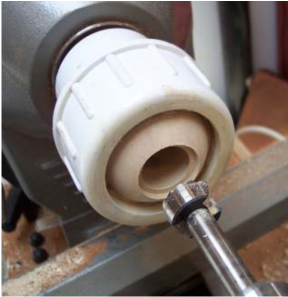
Photo 4. Drilling the 1" hole about ¾ of the way through the ball
