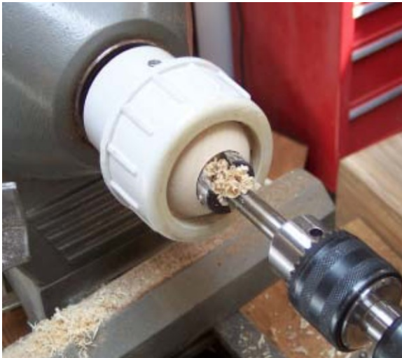
Photo 3. Drilling the 1-1/4" hole about 1/4" deep
