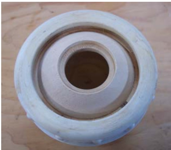
Photo 5. After hollowing the ball with a small offset tool
