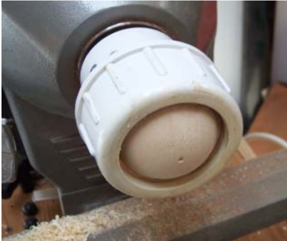
Photo 2. Ball held in ball chuck with center marked
