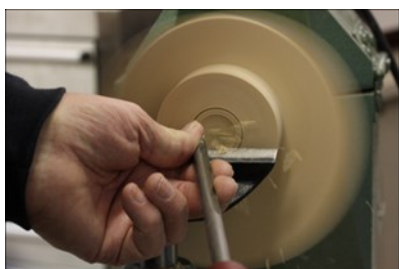
10. Turn a recess for the next scroll chuck mounting.
