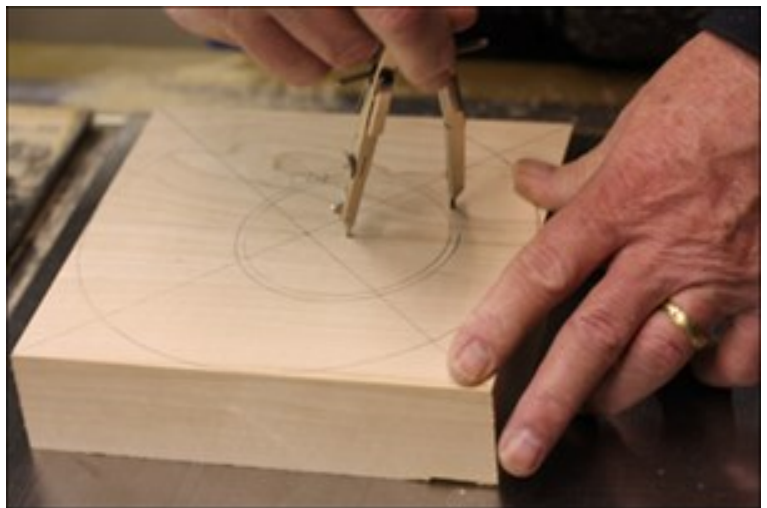
1. Lay out the design before mounting it to the lathe.
