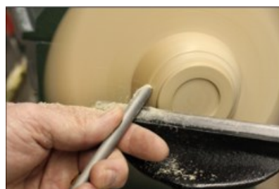
11. Form the foot and outside of the “bowl”. Sand to finished grit.
