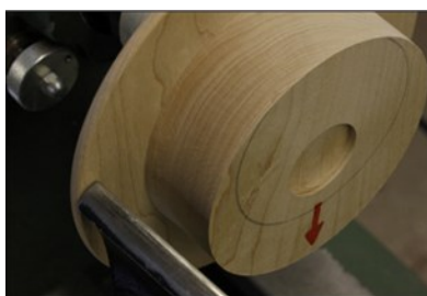
8. As the work rotates 90° (from photo 7) the distance to the tool rest increases. I recommend using a 5/8" or greater bowl gouge for this cut.
