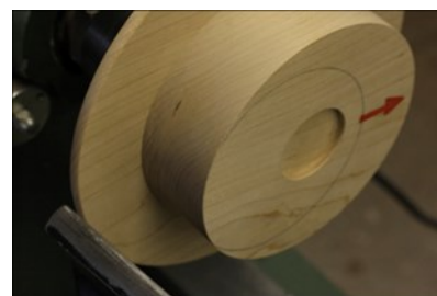
9. At 180° (from photo 7) the distance to the tool rest increases even more. This photo also shows the greatest amount of “air” you will be turning for this design.
