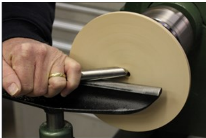
5. Flatten the top and finish the rim. Sand to finished grit.
