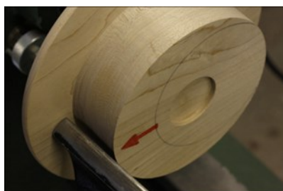
7. The distance from the tool rest to the blank will change as the blank rotates. Check your work before turning on the lathe.
