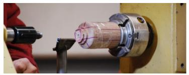
bottom together and back off the tail stock. Using light cuts finish cutting the top. Remove the bottom and install a jam chuck to fit into the opening of the box bottom and bring up tail stock. Using a parting tool or skew cut the tendon off the bottom and hand sand any nub.
