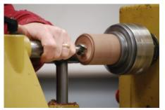
Box Lid Tool. He then sanded the inside and outside top edges. At this point you may sand the entire inside and outside of the box. Take care not to sand too fast or hard as it can heat up the wood and crack it.
