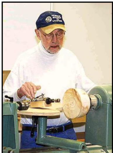
Jim's air powered die grinder & burr resting on "straight" fluting platform
