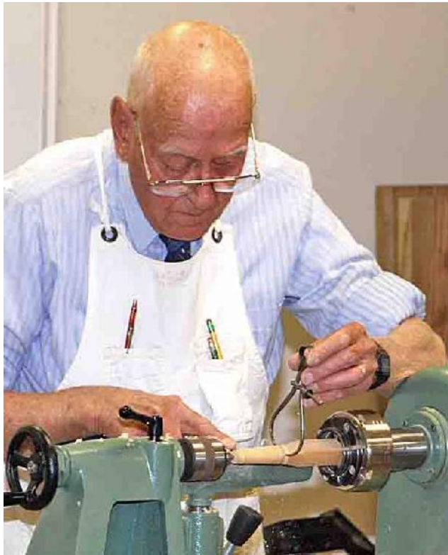
Bill uses calipers to gauge part
