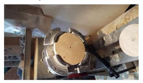
Set your compass to 3&1/2 inches. Mark each disk that you will be making coasters from, cut out using the band saw. Place between the friction drive and tailstock and turn away the saw marks.
