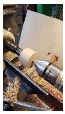
Place the blank into a small chuck, true up the tailstock side, drill a hole the size and depth for the BOC bead being used.
