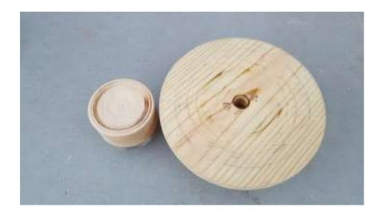
Place the wood that has been cut round on a bandsaw between the wooden disk and tailstock. I use the Hunter tools to true it up and also true the face towards the tailstock live center. You of course can use any tool of your choosing.
