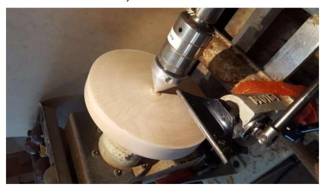
Using a compass, or dividers, mark a circle about 6 to 6&1/8". Remember to allow for fabric on the PVC, test the fit with the fabric glued onto the PVC. The grove can be from 1/8" to 1/4" deep depending on the thickness of the wood used. You will get a feel for this step as you progress along.
