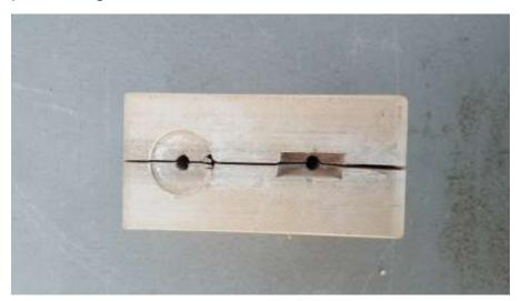
This is the completed Bead cutting Jig. Use a 1/8inch dowel or a skewer used for BBQing to hold the bead while cutting. Cut one side, turn the bead over and cut the other side. You will then need to smooth out the cut area. I use RTV to glue the bead into the top of the knob.
