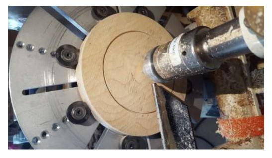
Back the tailstock away and remove the center disk.
