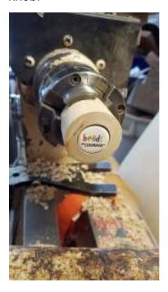
Form the top of the knob and sand using all the grits needed for a smooth finish.
