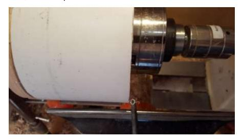
Stop the lathe, use a deburring tool to remove any frayed PVC both inside and outside. This can also be done with the PVC off the lathe. Do NOT use a deburring tool with the lathe running as it may grab the PVC.
