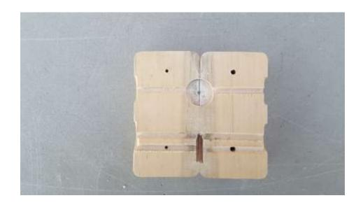
Place the two halves together as shown below. Clamp together and drill two 3/16 inch holes through the wood to assist with removing stuck beads when cutting.
