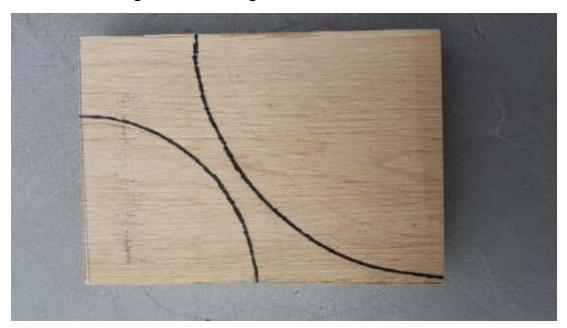
Use a compass and mark quarter circles, one for the Stronghold chuck 4&1/4 inches and the smaller quarter for the talon chuck at 3 inches as marked above. Do this on all four pieces of Maple stock.
