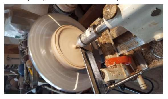
Back the tailstock away and remove the small nub.
