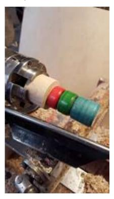
The picture below shows a cut bead in the wood which will be the top of the finished knob.
