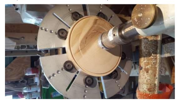
Test fit the PVC into the grove. Remember to allow for the fabric being used.
