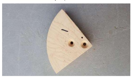
Mark jaws as drilled to be placed on the chuck.
