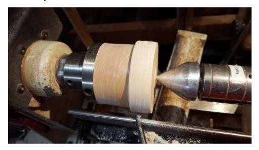
Place a disk into the chuck as pictured below with the plywood spacer behind the disk. Use a thin parting tool and cut the disk in half. See the picture below.
