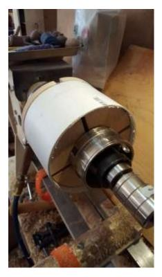
Turn on the lathe, about medium speed and carefully true up the end of the PVC pipe at the tailstock end. Stop the lathe, loosen up both chucks, turn the PVC around, tighten both chucks and again true up the PVC at the tailstock end. I use the Hunter #1 tool, see the picture below.
