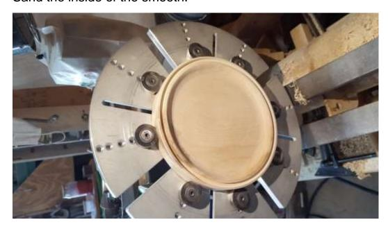
Turn the bottom around and finish the bottom as shown in the picture below. I like to put signature rings in the bottom.
