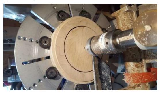
Turn the top disk around and cut through to the previous cut as in the picture below.
