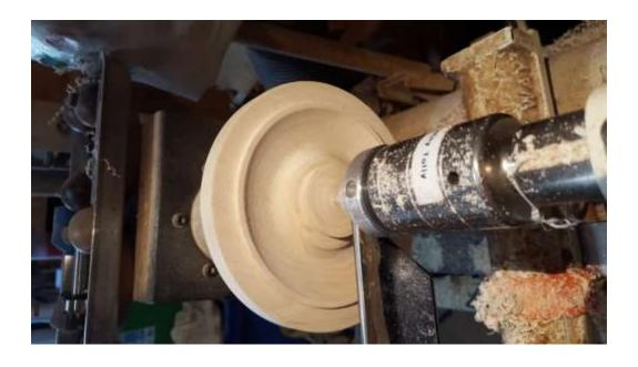
Test fit the lid as in the picture below. Here the wood is over sized and will be trimmed down to fit the top nicely in the next steps.
