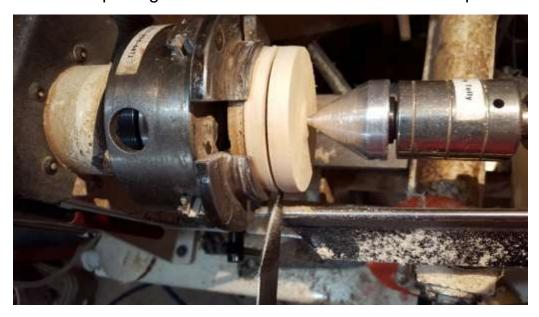
True up the face of the disk which is not completed in the picture below yet.
