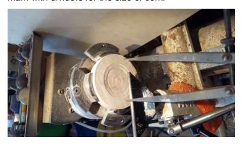
Turn the recess in the face of the disk, make sure that the cork fits and then sand the face smooth.
