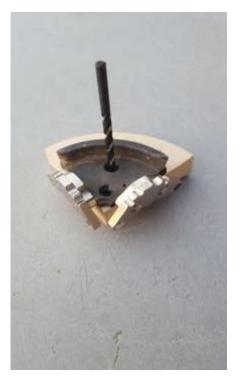
Counter sink all of the holes for the screws so that the screws will sit flush or below the surface of the wood being used.
