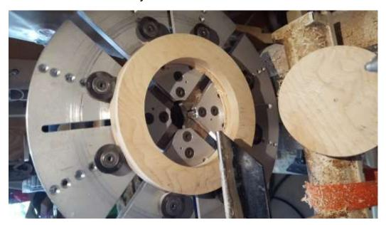
Put the Talon chuck with the wooden step jaws onto the headstock. See the picture below for the wooden step jaws.
