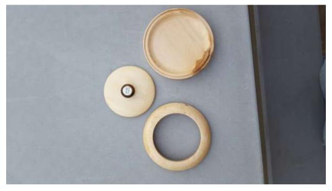
Note: I use regular Titebond II wood glue for gluing the knob into the top of the lid. I use Silicone RTV type sealant for the top and bottom grooves to hold the PVC and fabric.
