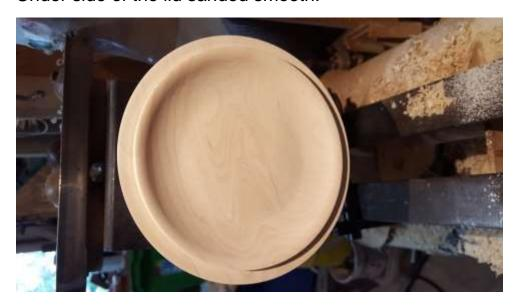
Note: I often use a vacuum system to turn the lid, both the inside and the outside. I will turn the lid around and undercut the lid reducing the weight. If not using a vacuum system, you may do one of the following.
