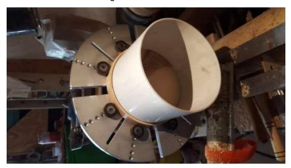
Thin down the inside of the bottom to make the BC box lighter. For safety, keep the tailstock up until just a small nub is left. See the picture below.
