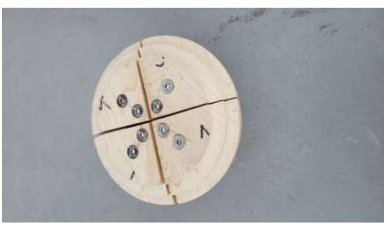
I have made much larger wooden jaws to hold the top and bottom pieces for the BOC boxes. You can do this if you do not have the Jumbo type aluminum jaws. Purchase 6mm T nuts for the back of the plywood and used the Oneway rubber pads.
