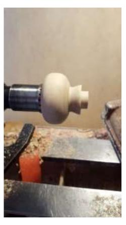
I made a simple go-no-go gauge to insure that the tennon is the correct size to mount into the lid. Use a forstner bit and small scrap of thin stock to make the go-no-go gauge.
