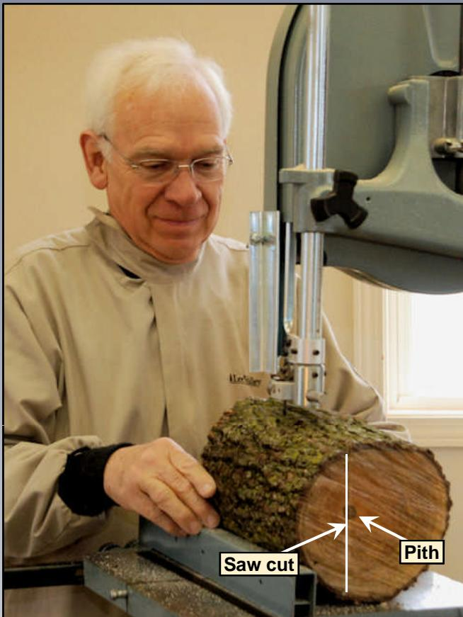
Cutting the log on a band saw.
