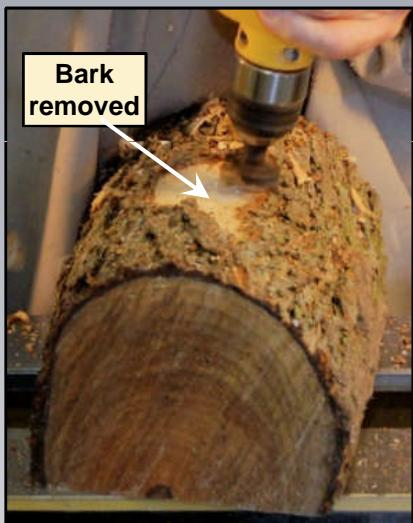
Remove a large enough area of bark to allow repositioning the drive center for bowl centering adjustment later. I use a stub drive center or 4-prong drive center.
