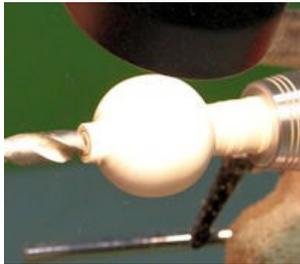
**Drilling the 9/16 hole<sup>1</sup>**
