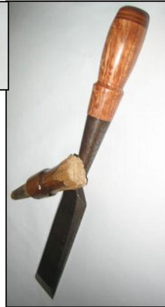
**New handle on refurbished chisel.**
