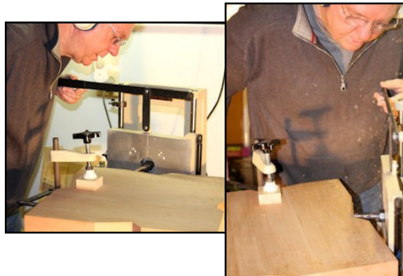
Two views of Bruce making the base side cuts on the Multi-Router.
