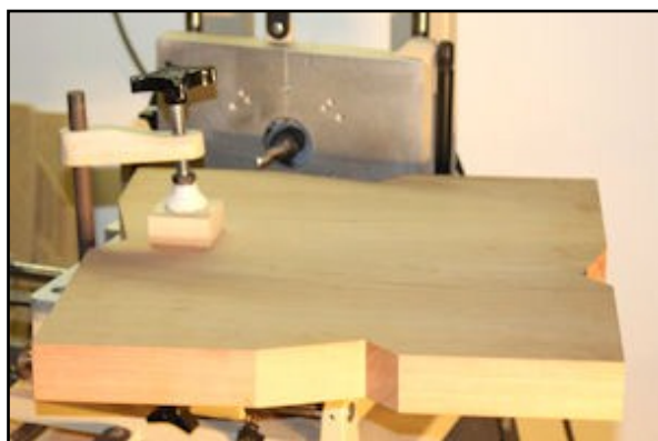
The base is set up on the Multi-Router for a side cut detail.
