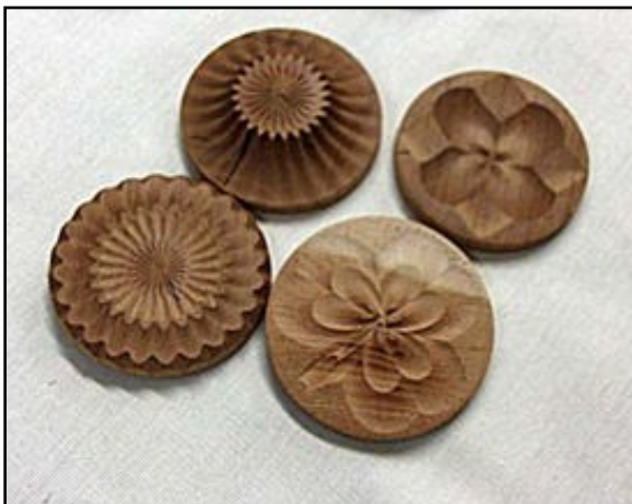
(Fig. 4) Examples of surface contours and shapes that can be made with the rose engine lathe.
