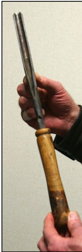
Bill McColgin's old bowl gouge, made from a file. The close up detail shows remnant file teeth on the reverse side of the gouge.
