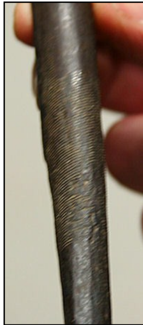
Bill McColgin's old bowl gouge, made from a file. The close up detail shows remnant file teeth on the reverse side of the gouge.
