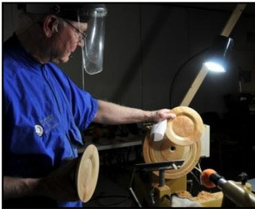
Cut away the tenon with pull cuts as on the front. The new cut on the bottom is transitioned with the old cut in the area before the rise to the foot. The transition is better hidden on the flat. Pull shear scraping with the sweptback gouge is again followed by the skew. The bottom doesn't have to be perfectly flat really. Just another tip; if making a plate from a board, where surplus material isn't available, glue a waste block on for the tenon.
