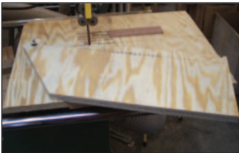
The two pieces have been attached to one another with a pivot bolt and are ready to make the saw cut into the swinging board.
