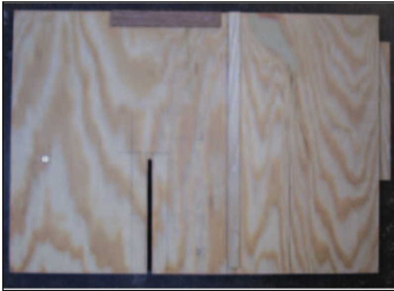
Bottom side of the base board for the circle cutting jig.
