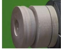
Add texturing if desired and if adding a cabochon, make an indent with the skew to center the drill for cutting a 1/16" recess. The key is to make both sides identical. Last, finish cutting the string section, which was only ½" deep, to give a 3/8" diameter spindle.
