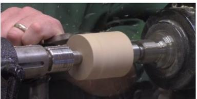
ideally be between 45 and 75 g. Orientation of the grain is critical. If the grain runs perpendicular, the spindle will snap. Jeff holds the work in a scroll chuck and uses o-rings to hide the dovetails. The o-ring must be under 2"" in OD. Jeff uses a #132, available from a supply house like McMaster-Carr or some local hardwares. Durometer hardness can range from about 50 to 70. Silicone (red rubber) runs 50. Jeff doesn't like
