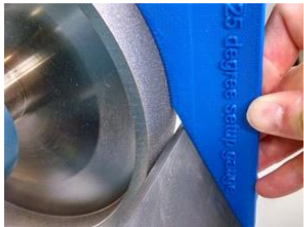
One of many grinder jigs found on Thingiverse This jig may be found Here
